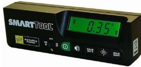
The Smarttool GEN3 can measure all angles in a 360 degrees range.
